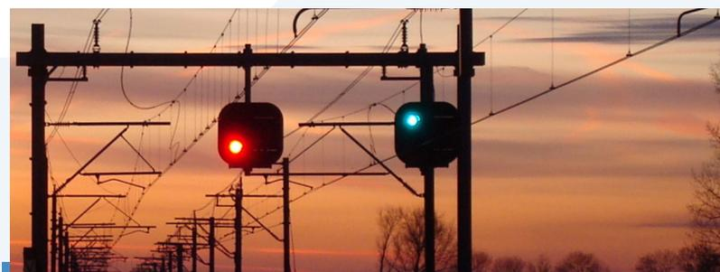
AY signals can be mounted on posts and gantries. Post-mounted signals can be supplied with platform and ladder, and can also be supplied in combination with a Matrix Signal Generator (MSGw2).
